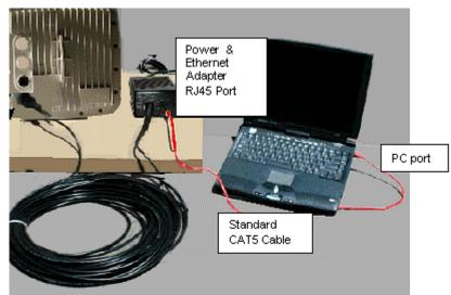
WARNING! The maximum length of the CAT 5 cable allowed between the radio unit and the power & Ethernet adapter is 75 meters. If you are connecting the radio through a hub or switch, the maximum length of the two CAT 5 cables is 75 feet; for example, if the cable between the radio and the power supply is 50 feet, the cable between the power & Ethernet adapter and the PC can be only 25 feet, for a total length of 75 feet.
